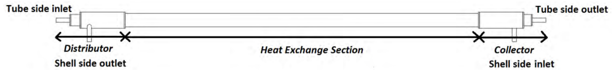
Fig. 6.1. Side view of the multi-tube mini-channel heat exchanger. Shell side internal diameter is 21 mm.
