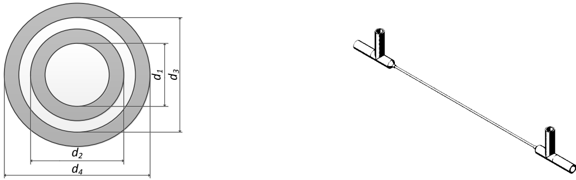
Fig. 4.2. Left: Mini-channel cross-sections. Light gray is the flow area; dark grey is the wall. Right: 3D drawing of 1.1x200 mm inside diameter tube including the shell tube with 2.5 mm external diameter. For the annulus under consideration, d_1 = 1.1 mm, d_2 = 1.6 mm, d_3 = 2.0 mm and d_4 = 2.5 mm. The heat exchanger is insulated with heat resistant foam to prevent heat loss to the ambient.
