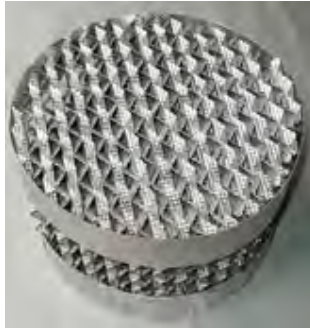
Figure 3.4. Structured packing (Mellapak 250 Y) for the acid wash column with a diameter of 0.65 m and a height of 0.22 m for each layer.
