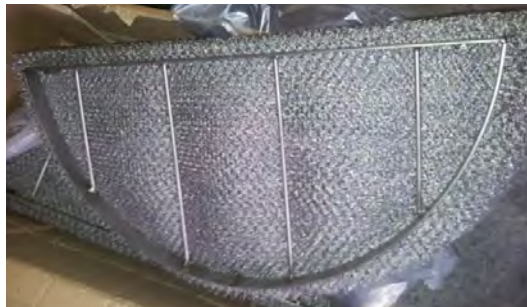
Figure 3.6. Conventional knit mesh demister for droplet removal with a diameter of 0.65 m and a height of ca. 10 cm.
