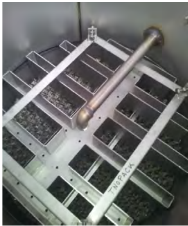
Figure 3.5. Liquid distributor over the structured packing in the acid wash column. It has a diameter of 0.65 m and the total number of orifices are 50, each with a diameter of 7.1 mm.
