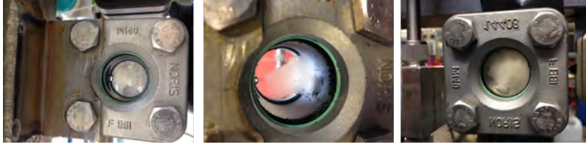
Figure 5.5: Hydrate formation periods. Left: before hydrates appear; Center: In the middle of hydrate formation; Right: Blockage in the end of hydrate formation.
