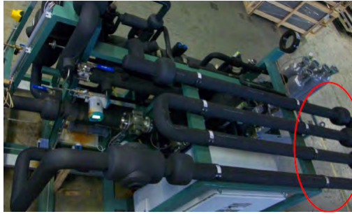
Figure 4.4: Static mixer tubes of pilot plant. The red cycle shows that there are four tubes connected in series. The static mixer is needed to ensure a well-mixed water-CO 2 solution.
