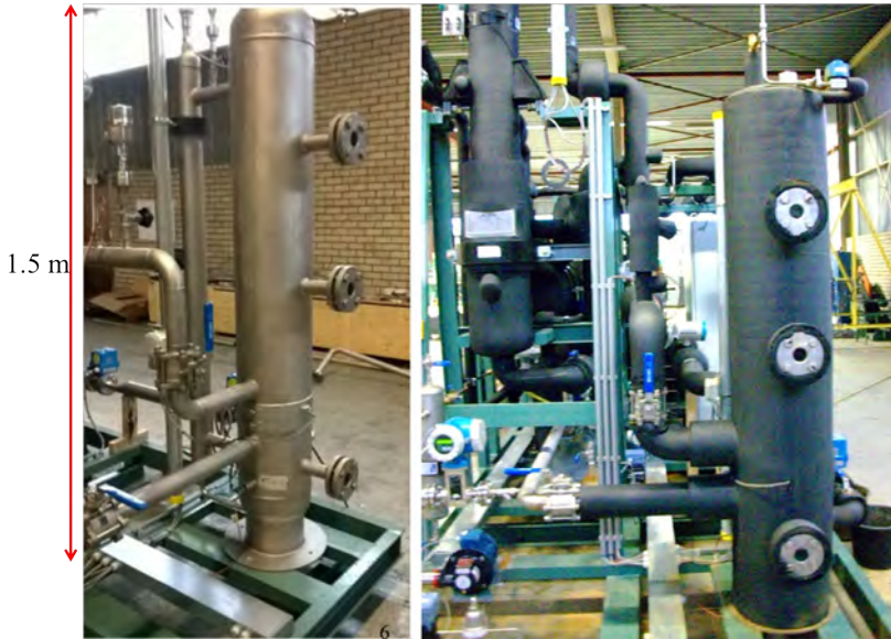
Figure 4.3: Picture of the cold storage vessel before (left) and after (right) being insulated showing the position of the three sight glasses.
