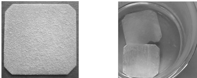
Figure E.8: Photographs of CAU-10-H synthesized directly on m-Al (without pretreatment) using standard conditions (SSP) ( left ) and with addition of 2 g \text{Al}_2(\text{SO}_4)_3 \cdot 18\text{H}_2\text{O} ( right ).
