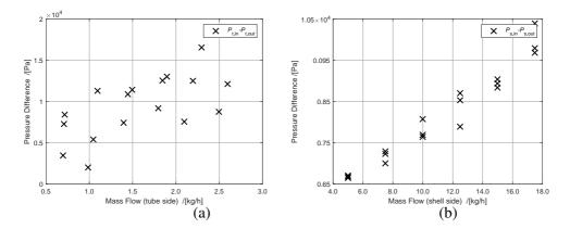
Figure 3.15: Pressure drop over the mini-channel heat exchanger on the tube side (NH<sub>3</sub>-H<sub>2</sub>O side) (a), and the shell side (water side) (b).
