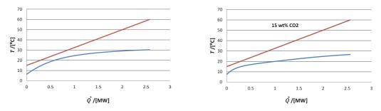
Figure 2.17: Temperature profiles in the desorber as a function of the heat load. Left: profiles for the ammonia water mixture. Right: added CO<sub>2</sub> (15 wt%) calculated with the new fit.
