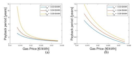
Figure 5.10: The simple payback period as a function of the gas and electricity price for a compressor outlet vapor quality of 0.5 and NH $_3$  concentration of 0.55, when waste heat stream is heated from 90 to 130  $^{\circ}$ C, assuming 5 MW thermal output. Not taking into account the cost of CO $_2$  (a), taking into account the cost of CO $_2$  (b)
