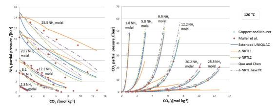
Figure 2.3: Comparison of the experimental data from Göppert and Maurer [44] and Müller et al. [45] for partial bubble point pressures of  $CO_2$  and  $NH_3$  at 120 °C with the model correlations.
