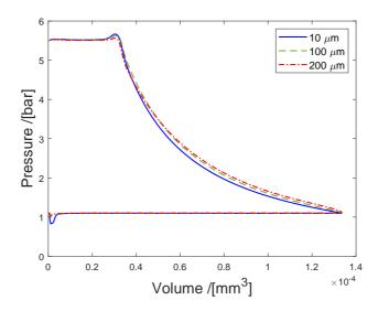
Figure 4.5: *P-V* diagram for 10  $\mu$ m (blue solid line), 100  $\mu$ m (green dashed line) and for 200  $\mu$ m (red dash-dot line).
