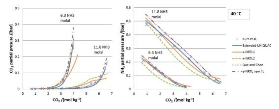
Figure 2.2: Comparison of the experimental data from Kurz et al. [27] for partial bubble point pressures of  $CO_2$  and  $NH_3$  at 40 °C with the model correlations.
