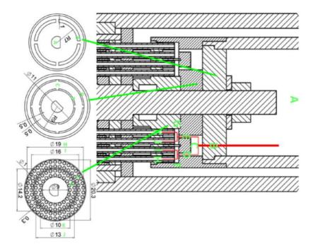
Figure 3.2: Illustration of the fractal distribution that is used both on tube and shell sides of the mini-channel heat exchanger to guarantee pure counter current flow of the heat exchanger fluids [74]. The bottom left figure shows how the tubes are arranged in the shell of the heat exchanger. Dimensions are in mm.
