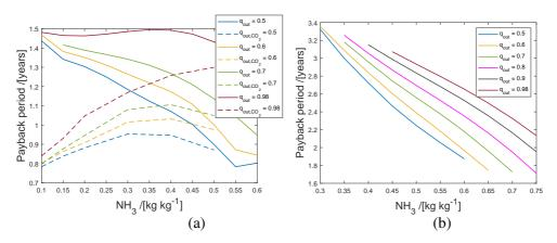
Figure 5.7: The simple payback time taking the cost of  $CO_2$  into account as a function of the  $NH_3$  concentration for various compressor outlet vapor qualities, assuming 5 MW thermal output, when a waste heat stream is heated from 90 to 130 °C (a) and from 60 to 140 °C (b). The solid lines are the results for  $NH_3$ - $H_2O$  and the dotted lines with added 5 wt%  $CO_2$ .
