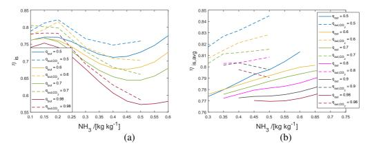
Figure 5.3:  $\eta_{is}$  as a function of the NH<sub>3</sub> concentration for various compressor outlet vapor qualities when a waste heat stream is heated from 90 to 130 °C (a) and from 60 to 140 °C (b). The solid lines are the results for NH<sub>3</sub>-H<sub>2</sub>O and the dotted lines with added 5 wt% CO<sub>2</sub>.
