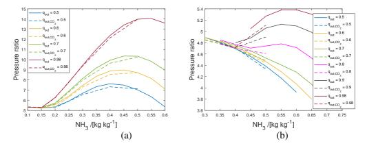
Figure 5.2: Pressure ratio as a function the  $NH_3$  concentration for various compressor outlet vapor qualities when a waste heat stream is heated from 90 to 130 °C (a) and from 60 to 140 °C (b). The solid lines are the results for  $NH_3$ - $H_2O$  and the dotted lines with added 5 wt%  $CO_2$ .
