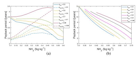
Figure 5.5: The simple payback time as a function of the  $NH_3$  concentration for various compressor outlet vapor qualities, assuming 1 MW thermal output, when a waste heat stream is heated from 90 to 130 °C (a) and from 60 to 140 °C (b). The solid lines are the results for  $NH_3$ - $H_2O$  and the dotted lines with added 5 wt%  $CO_2$ .
