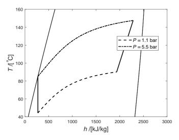
Figure 4.3: *T-h* diagram of a CRHP, using wet compression, for 30 wt.% NH<sub>3</sub>. The compression process is entirely in the two phase region from the lower to the higher pressure level. The resorption happens at the higher pressure level, 5.5 bar in this case, then isenthalpic expansion is assumed and the desorption process is at 1.1 bar.
