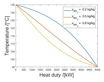
Figure 5.9: Example temperature glides as a function of the heat load for NH<sub>3</sub> concentrations of 0.2 kg/kg, 0.5 kg/kg and 0.8 kg/kg.
