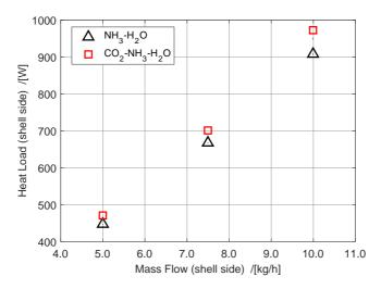
Figure 3.18: Shell side heat load for the NH<sub>3</sub>-H<sub>2</sub>O and NH<sub>3</sub>-CO<sub>2</sub>-H<sub>2</sub>O experiments.
