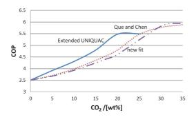
Figure 2.15: COP vs CO<sub>2</sub> weight fraction, 0.3 to 25 bar pressure limit; waste heat stream is heated from 60 to 105 °C. Results from the extended UNIQUAC model are shown with continuous line, the model of Que and Chen [33] with dotted line, and the new fit with dashed line.
