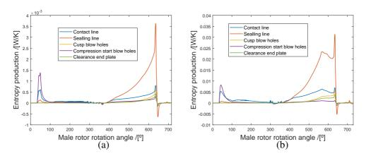
Figure 4.4:  $\dot{\sigma}$  for each leakage path in the compressor, 10  $\mu$ m (a) and 100  $\mu$ m (b).
