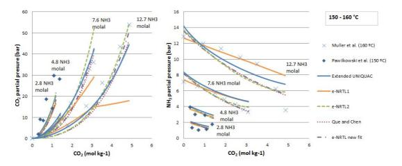
Figure 2.4: Comparison of the experimental data from Müller et al. [45] and Pawilkowski et al. [50] for partial bubble point pressures of  $CO_2$  and  $NH_3$  at 150 °C and 160 °C with the model correlations.
