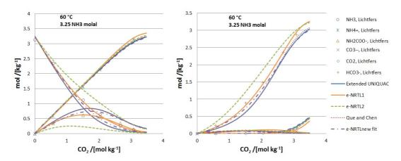
Figure 2.7: Comparison of the experimental data from Lichtfers [53] for speciation at  $60 \, ^{\circ}\text{C}$  and molality of 3.25 mol/kg NH<sub>3</sub> with the model correlations.
