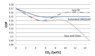
Figure 2.16: COP vs CO<sub>2</sub> weight fraction, cooling case; waste heat stream is heated from 60 to 105 °C and partially cooled down to 15 °C. Results from the extended UNIQUAC model are shown with continuous line; the model of Que and Chen [33] with dotted line, and the new fit with dashed line
