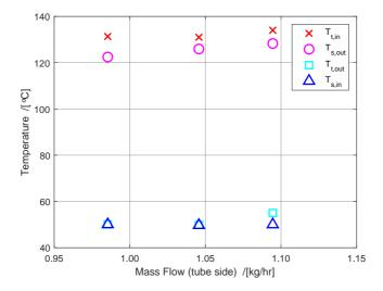
Figure 3.11: In- and outlet temperatures for the  $NH_3$ - $H_2O$  experiments at various tube side mass flows when the shell side mass flow is kept constant at 7.5 kg/h.
