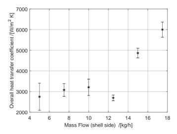
Figure 3.13: The overall heat transfer coefficient for the optimum tube side mass flows of the  $NH_3$ - $H_2O$  experiments.
