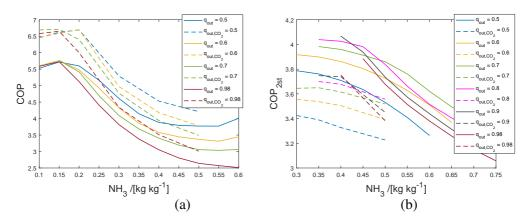
Figure 5.1: COP as a function of the  $NH_3$  concentration for various compressor outlet vapor qualities when a waste heat stream is heated from 90 to 130 °C (a) and from 60 to 140 °C (b). The solid lines are the results for  $NH_3$ - $H_2O$  and the dotted lines with added 5 wt%  $CO_2$ .
