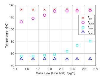
Figure 3.16: The in- and outlet temperatures for the NH<sub>3</sub>-CO<sub>2</sub>-H<sub>2</sub>O experiments at various tube side mass flows when the shell side mass flow is kept constant at 5 kg/h.
