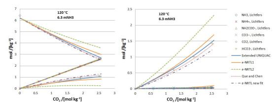
Figure 2.8: Comparison of the experimental from Lichtfers [53] data for speciation at  $120\,^{\circ}$ C and molality of 6.3 mol/kg NH<sub>3</sub> with the model correlations.
