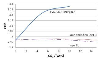
Figure 2.18: COP vs CO<sub>2</sub> weight fraction, cooling included and 0.3 bar lower pressure limit. Results from the extended UNIQUAC model are shown with continuous line; the model of Que and Chen [33] with dotted line, and the new fit with dashed line.
