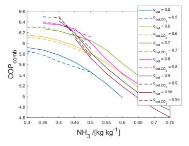
Figure 5.4:  $COP_{comb}$  as a function of  $NH_3$  concentration for various compressor outlet vapor qualities when a waste heat stream is heated from 60 to 140 °C. The solid lines are the results for  $NH_3$ - $H_2O$  and the dotted lines with added 5 wt%  $CO_2$ .
