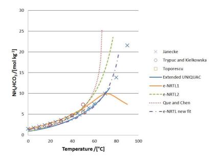
Figure 2.6: Comparison of the experimental data from Janecke [43], Trypuc and Kielkowska [51] and Toporescu [52] for solubility of NH<sub>4</sub>HCO<sub>3</sub> in water with the model predictions.
