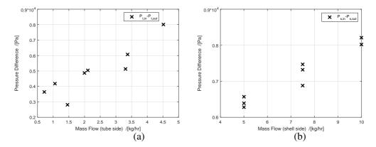
Figure 3.17: Pressure drop over the mini-channel heat exchanger on the tube side ( $NH_3$ - $CO_2$ - $H_2O$  side) (a), and the shell side (water side) (b).
