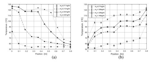
Figure 3.23: Temperature values along the mini-channel for a shell side mass flow of 5 kg/h, for downward absorption of the NH<sub>3</sub>-CO<sub>2</sub>-H<sub>2</sub>O mixture (a), and upward absorption of the NH<sub>3</sub>-CO<sub>2</sub>-H<sub>2</sub>O mixture (b). Error bars are included (see section 3.2 for details). The lines serve as visual guidelines for the reader.
