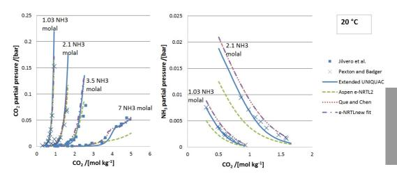
Figure 2.1: Comparison of the experimental data from Pexton and Badger [48] and Jilvero et al. [49] for partial bubble point pressures of CO<sub>2</sub> and NH<sub>3</sub> at 20 °C with the model correlations.
