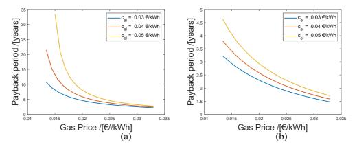
Figure 5.11: The simple payback period as a function of the gas and electricity price for a compressor outlet vapor quality of 0.6 and NH $_3$  concentration of 0.65, when waste heat stream is heated from 60 to 140  $^{\circ}$ C, assuming 5 MW thermal output. Not taking into account the cost of CO $_2$  (a), taking into account the cost of CO $_2$  (b)
