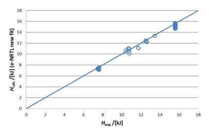
Figure 2.11: Comparison of the experimental data from Rumpf et al. [54] for heat of partial evaporation of the NH<sub>3</sub>-CO<sub>2</sub>-H<sub>2</sub>O mixture and the e-NRTL new fit correlation.
