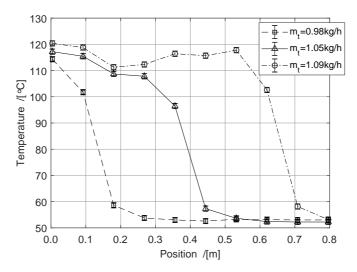
Figure 3.10: Temperature results from the sensors located along the shell side of the mini-channel heat exchanger when the shell side mass flow is fixed at 7.5 kg/h for the NH<sub>3</sub>-H<sub>2</sub>O experiments. Error bars are included (see section 2.2 for details). The lines serve as visual guidelines for the reader.
