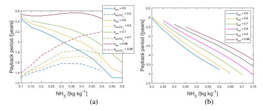
Figure 5.6: The simple payback time taking the cost of  $CO_2$  into account as a function of the  $NH_3$  concentration for various compressor outlet vapor qualities, assuming 1 MW thermal ouput, when a waste heat stream is heated from 90 to 130 °C (a) and from 60 to 140 °C (b). The solid lines are the results for  $NH_3$ - $H_2O$  and the dotted lines with added 5 wt%  $CO_2$ .
