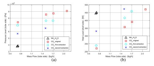
Figure 3.21: Results for a shell side mass flow of 5 kg/h before and after draining of the mixture with added  $CO_2$  compared to the NH<sub>3</sub>-H<sub>2</sub>O results, the different pressure levels (a), and the shell side heat load (b). It is clear that comparable pressure levels were not reached with the added  $CO_2$ . However, with each extraction the performance at similar mass flows approached the performance of the NH<sub>3</sub>-H<sub>2</sub>O mixture.
