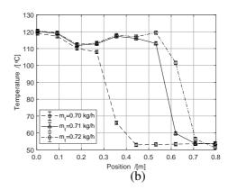
Figure 3.22: Temperature results from the sensors located along the shell side of the mini-channel heat exchanger for a shell side mass flow of 5 kg/h, for the NH<sub>3</sub>-CO<sub>2</sub>-H<sub>2</sub>O mixture (a), and the NH<sub>3</sub>-H<sub>2</sub>O mixture (b). Error bars are included (see section 2 for details). The lines serve as visual guidelines for the reader.
