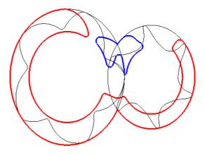
Figure 4.1: The twin screw compressor rotor profiles and shape of the radial suction port in red (there is also an axial suction port) and discharge port in blue.
