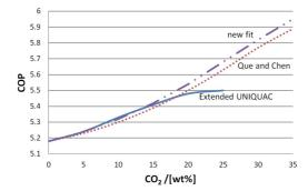
Figure 2.13: COP vs CO<sub>2</sub> weight fraction, heating case; waste heat stream is heated from 60 to 105 °C. Results from the extended UNIQUAC model are shown with continuous line, the model of Que and Chen [33] with dotted line, and the new fit with dashed line.
