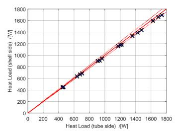
Figure 3.14: The heat load on the shell and tube sides for the  $NH_3$ - $H_2O$  experiments. The difference is within 3 % (dotted line) for all the experiments.
