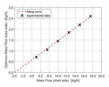
Figure 3.12: The optimum tube side mass flow for each shell side mass flow of the NH<sub>3</sub>-H<sub>2</sub>O experiments. A clear linear trend can be seen.
