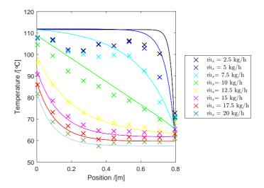
Figure 3.9: Temperatures along the length of the heat exchanger for the water-water experiments. Solid lines are calculated temperatures of the shell side flow with the method proposed by Nefs et al. [74], that is described above, and the marker values are from the temperature sensors along the heat exchanger.
