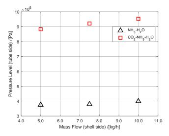
Figure 3.20: Pressure levels for the  $NH_3$ - $H_2O$  and  $NH_3$ - $CO_2$ - $H_2O$  experiments for shell side mass flows of 5, 7.5 and 10 kg/h.
