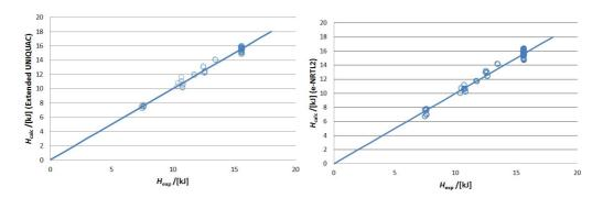
Figure 2.10: Comparison of the experimental data from Rumpf et al. [54] for heat of partial evaporation of the NH<sub>3</sub>-CO<sub>2</sub>-H<sub>2</sub>O mixture: (left) extended UNIQUAC and (right) e-NRTL2 correlation.
