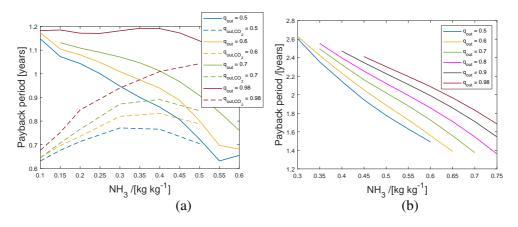
Figure 5.8: The simple payback time taking the cost of  $CO_2$  into account as a function of the  $NH_3$  concentration for various compressor outlet vapor qualities, assuming 10 MW thermal output, when a waste heat stream is heated from 90 to 130 °C (a) and from 60 to 140 °C (b). The solid lines are the results for  $NH_3$ - $H_2O$  and the dotted lines with added 5 wt%  $CO_2$ .
